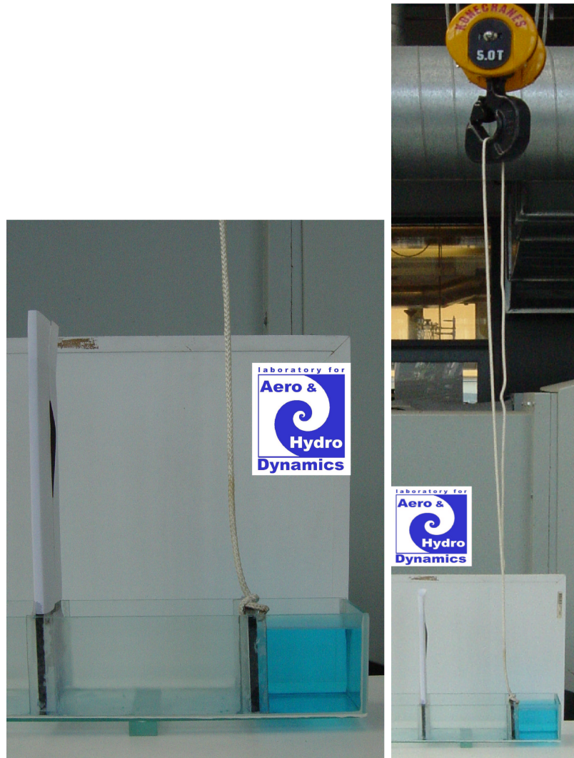
Figure 6.33: Dam breaking experiment set up (left) and manual pulley system to “instantaneously” remove the sluice gate (right).
