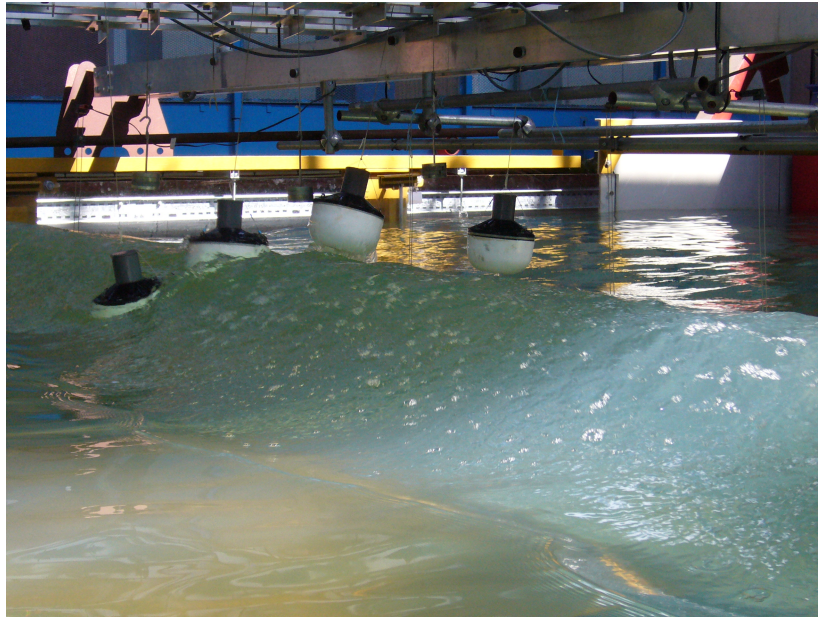
Figure 7.1: Physical tank with four floats in extreme waves
