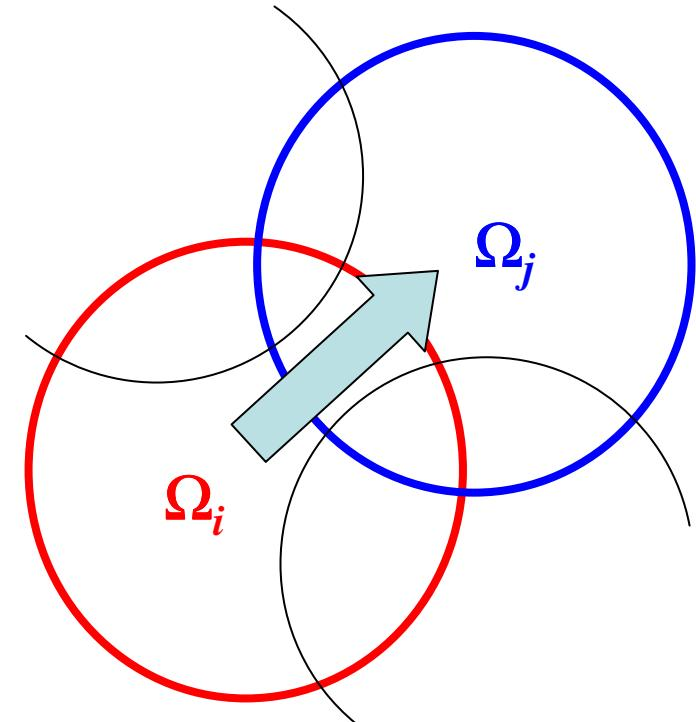
$$\int_{\Omega} \psi_i \frac{\partial \mathbf{U}}{\partial t} d\mathbf{x} - \sum_j \int_{\Omega} (\gamma_{ij} - \gamma_{ji}) \cdot \mathbf{F}(\mathbf{U}) d\mathbf{x} = 0$$
