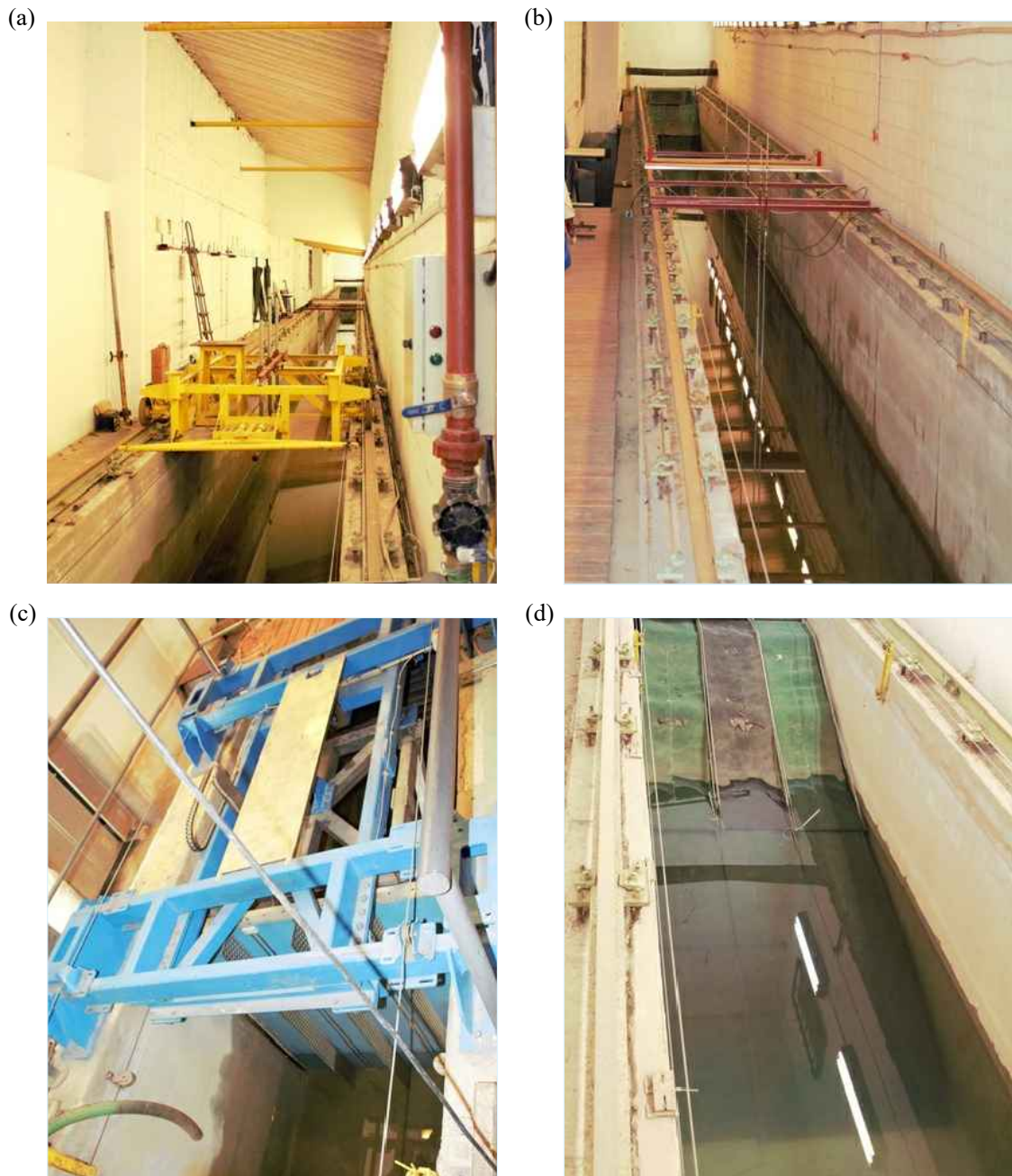
Figure 5.2: Wave flume: (a) full view; (b) measured section; (c) wavemaker; (d) beach.
