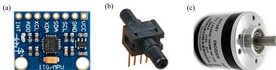
Figure 5.6: Experimental equipment: (a) integrated 6-axis motion tracking device; (b) pressure sensor; (c) encoder.
